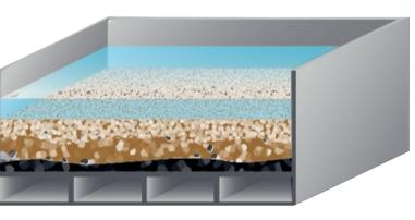
At the clarification stage (filter influent), turbidity is measured in order tomonitor the coagulation/ flocculation efficiency. Higher turbidity levels would lead to faster clogging of the filters, which in turn leads to wasting more water to backwash filters and higher power consumption.
