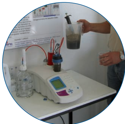
Fig. 1: The TIM 840 titrator for FOS/TAC determination at the Wambeln biogas plant.
